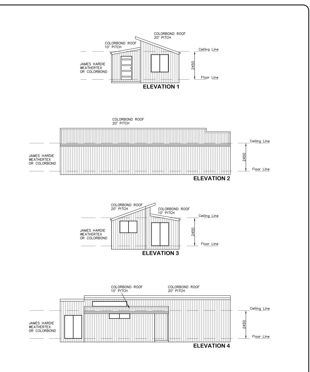
\* ALL DIMENSIONS ARE TO BE CONFIRMED BY THE BUILDER PRIOR TO CONSTRUCTION. DO NOT SCALE FROM DRAWINGS. BUILDING SET OUT & SITE BOUNDARY DETAILS TO BE CONFIRMED BY A REGISTERED SURVEYOR. ALL WORK TO BE CARRIED OUT TO RELEVANT STANDARDS AND BUILDING CODES.
